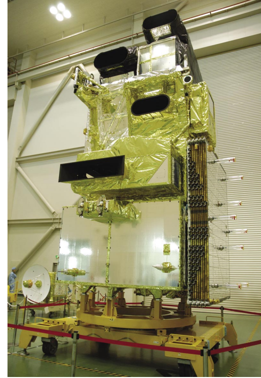
“Advanced Land Observation Satellite” (ALOS): This satellite, which is also called “Daichi” by the Japan Aerospace Exploration Agency JAXA, is used for precise land coverage observation. It was successfully launched in January 2006 and is an example of the perfect interaction of hardware and software in a critical application area. Photo ©JAXA
