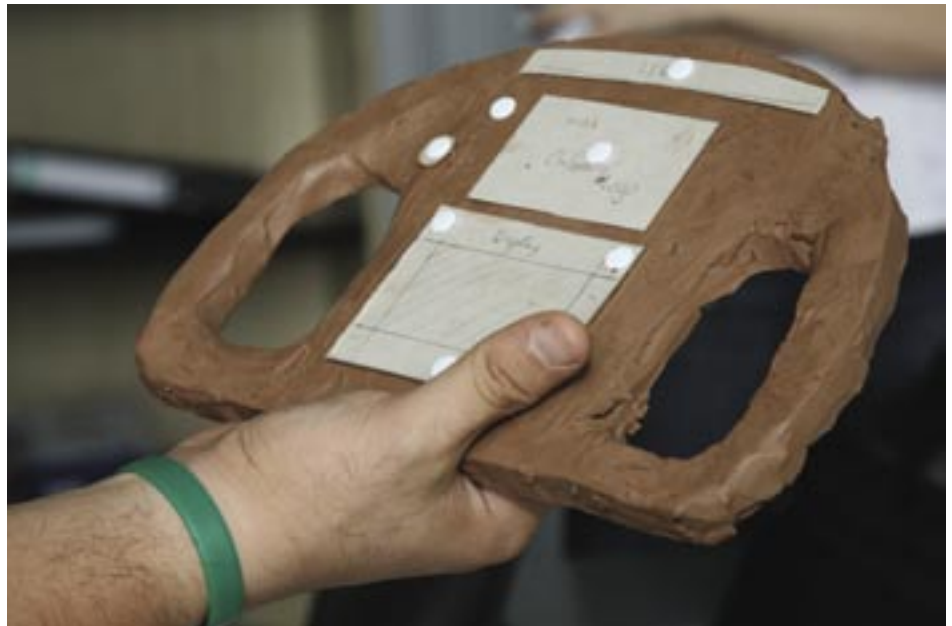
Design study: So far, the steering wheel only exists as a clay model – the control and display elements are already in place.
